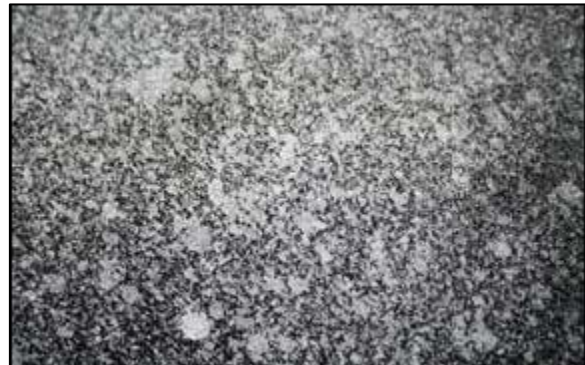
FIGURE 4-2 AN EXAMPLE OF INSUFFICIENT PRETREATMENT
