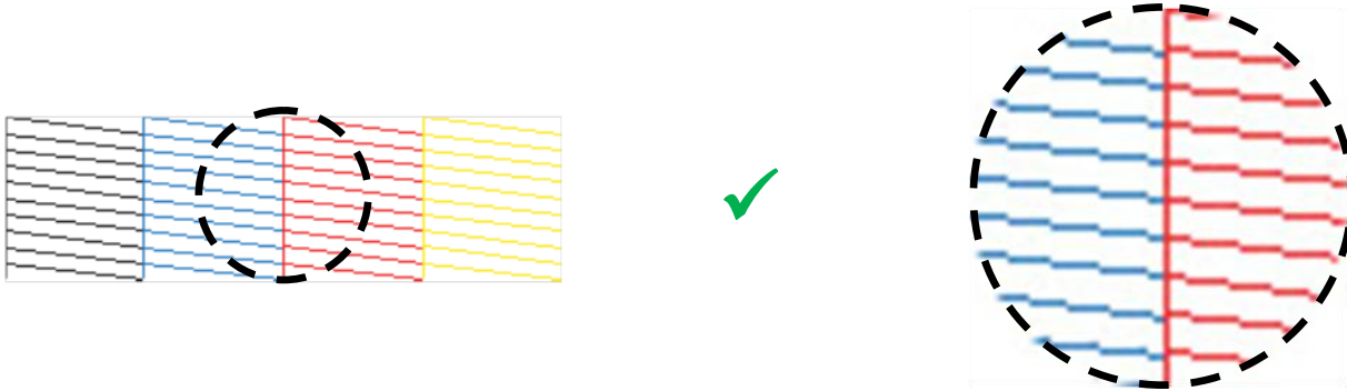
FIGURE 3-5 GOOD NOZZLE TEST PRINT
